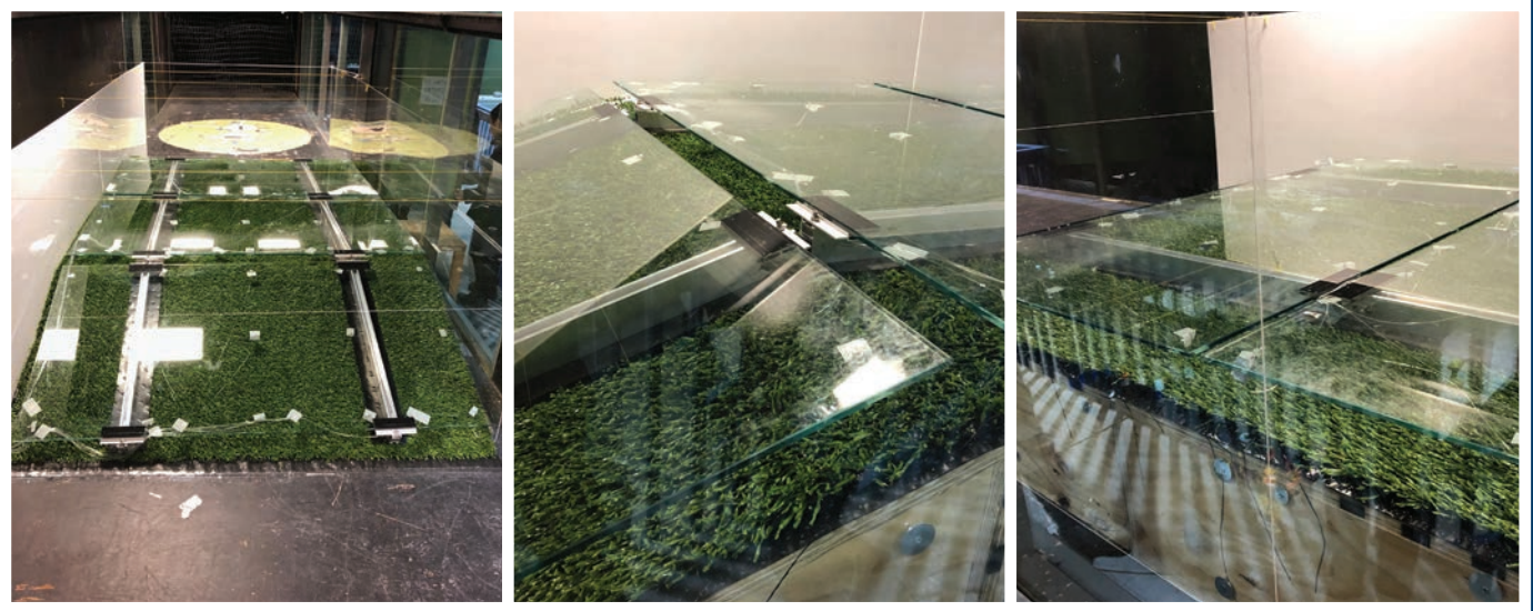
Wind Tunnel testing of ClosureTurf® and PowerCap™
